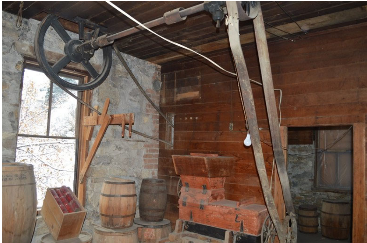
MT_LewisAndClarkCounty_Shaw'sBestFactory_0013 of 0020: Shaw's Best Factory. Second floor interior, east residential/production room, west wall, Hunter Lightning Sifter/Mixer and rotator shaft, pulleys and belts looking southwest.
