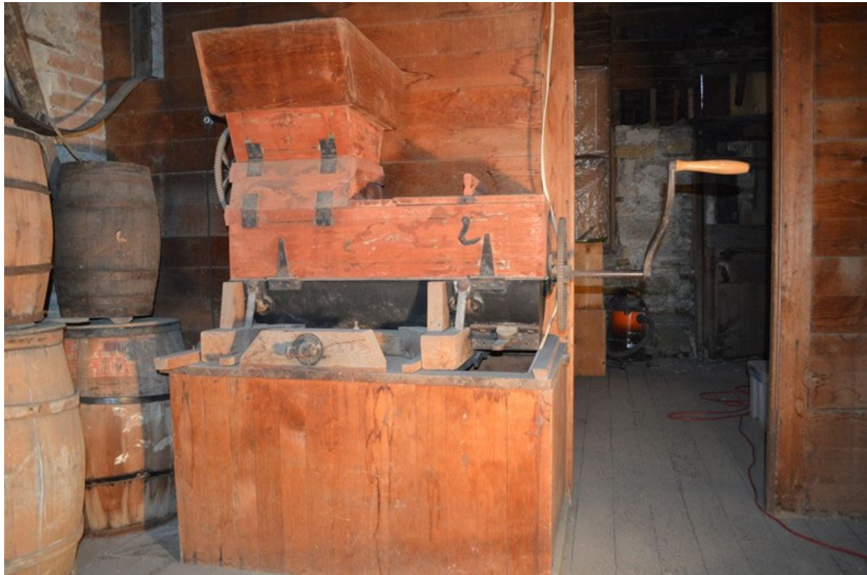
MT_LewisAndClarkCounty_Shaw'sBestFactory_0012 of 0020: Shaw's Best Factory. Second floor interior, east residential/production room, west wall, Hunter Lightning Sifter/Mixer looking west.
