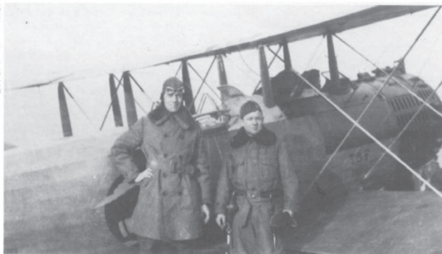
Jack Milburn, left, with observer Dell H. McCoy of Miller, South Dakota. McCoy wears the belt hooks that attached to the tourelle during flight, and held the observer in his cockpit.
