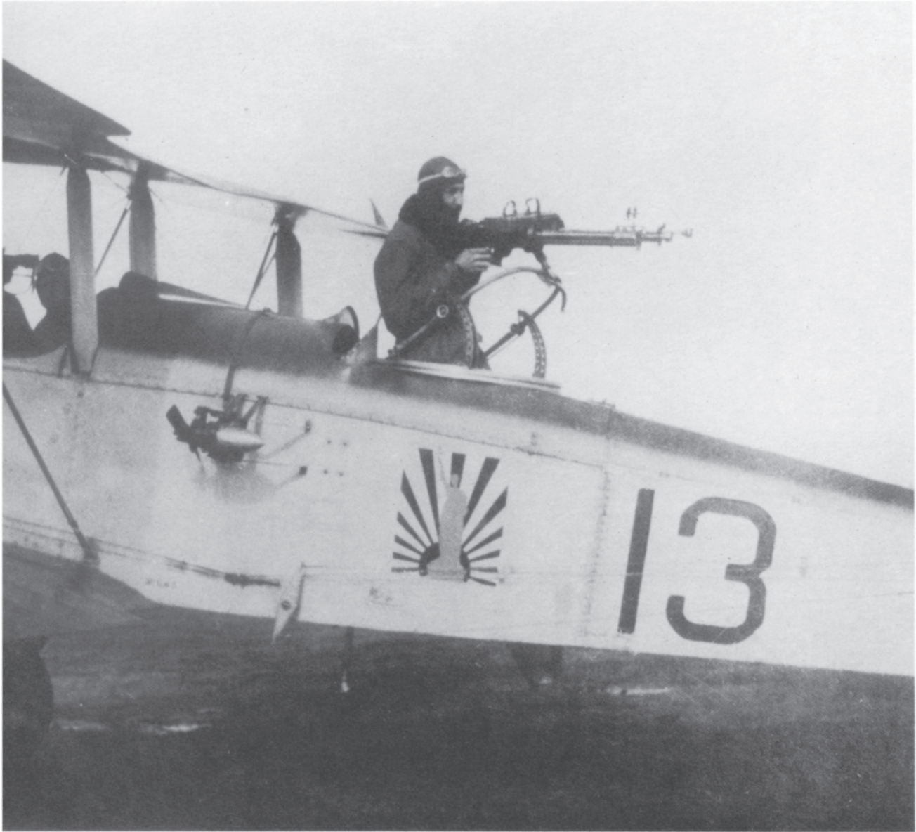
Bill Belzer poses in the observer's fighting position: standing inside the tourelle, Lewis gun at the ready. To right of wings, note small propeller of the wind-driven plate-changing mechanism for the camera.
