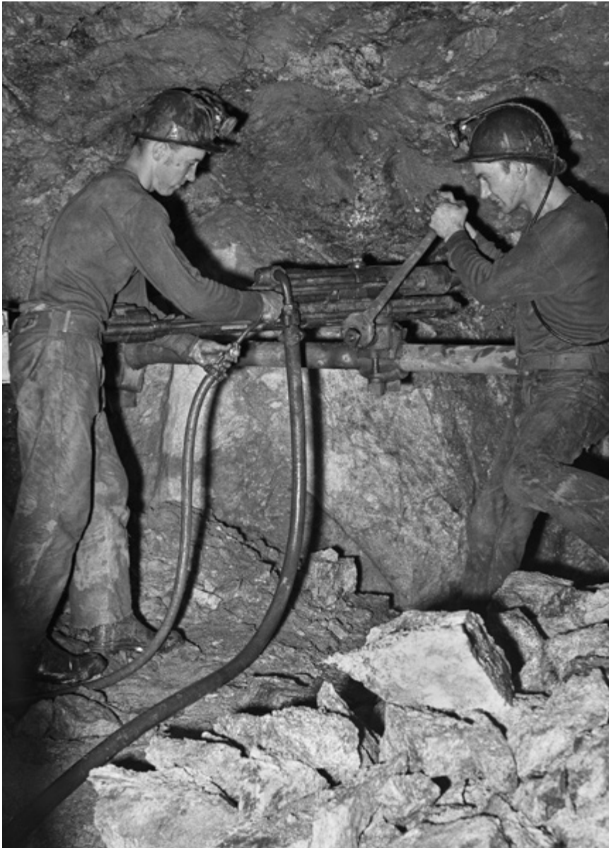
These underground miners, identified as Schmooke and Larson, are “setting up a drifter” to drill holes to fill with dynamite and blast the rock loose. They may have been working as stope miners, “the ones that went up and broke the rock and cut it down,” according to Steve Sherick, or as drift miners—“the ones that dig the tunnels” (also called drifts).
