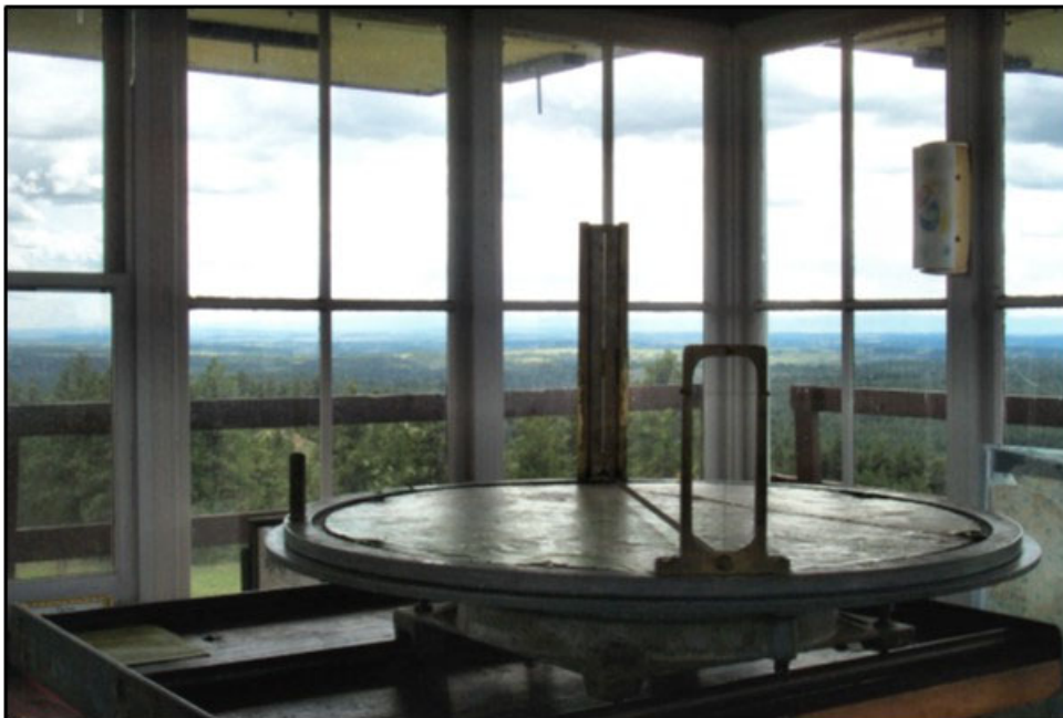
MT_RosebudCounty_PokerJimButteLookout_0005. Looking across the Osborne Firefinder from inside the structure, Site 24RB2233, Poker Jim Butte Fire Lookout May 17, 1999, View to Southwest (Urbaniak 1999)
