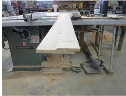
Figure 9: Harding House Exterior - siding re-fabrication
