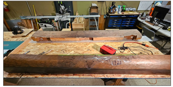
Jacob Franklin traced the brands, then hand scribed them to the wood surface. The branding was mimicked with an electric wood burner.
